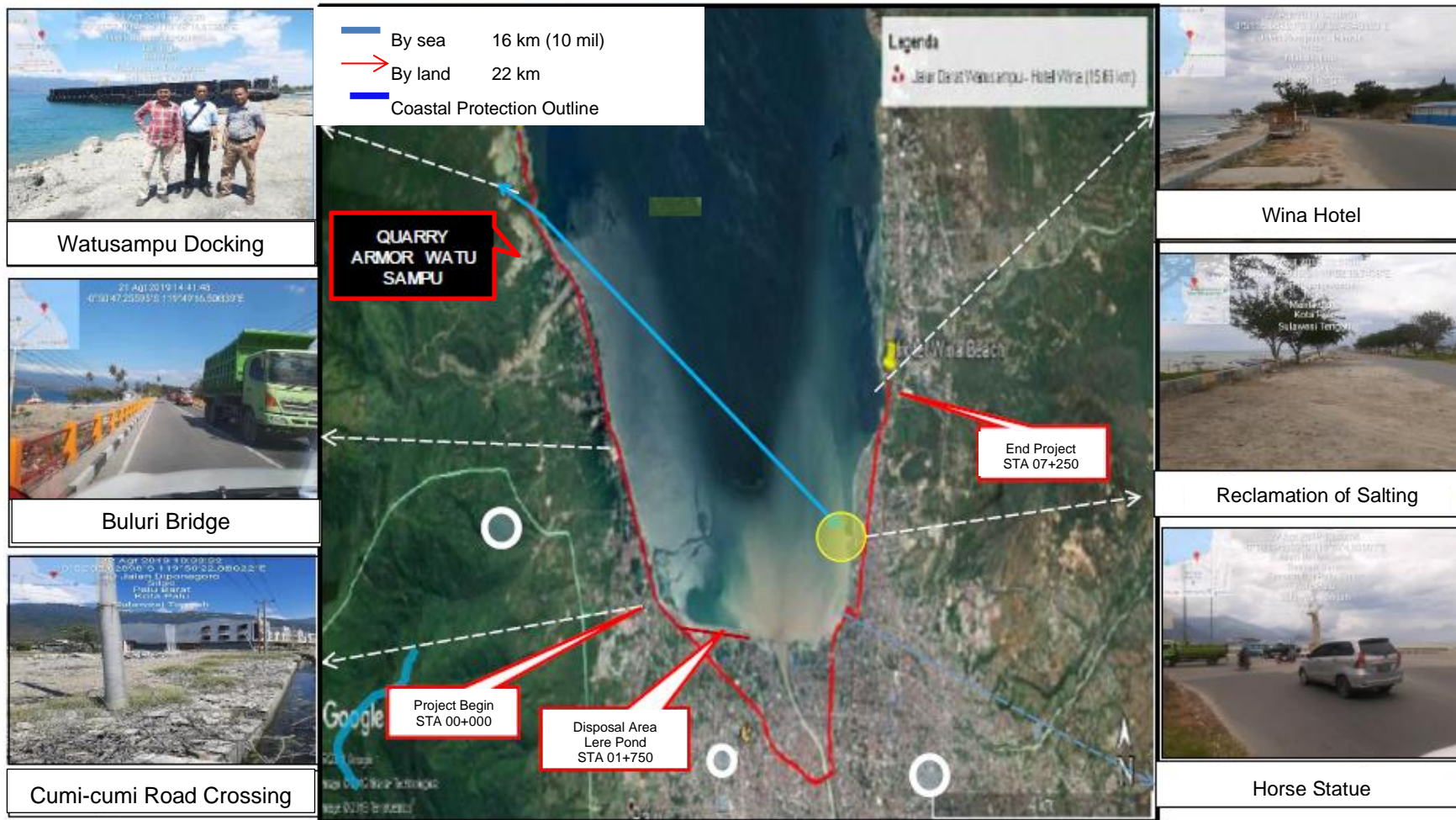
Figure 6: Material path from the quarry to the project site and disposal site
